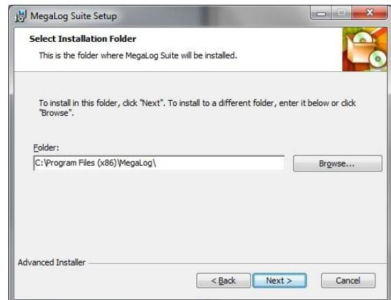
The installer is now ready to install all three services, documentation, tools and the presentation module. The database will be created automatically after the first start of service DBMaintenance (~ after one minute).
